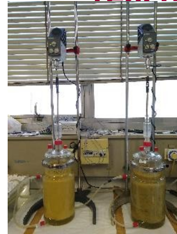
Operating at 35°C and 3.5/5d of HRT, pH6/7, with and without compost addition
